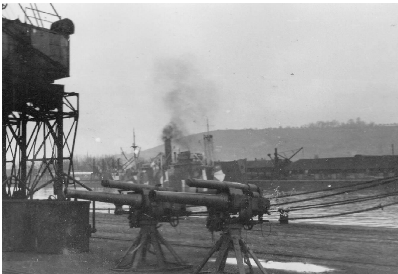
Two 90 mm French Mle 1877 guns converted on the naval mounts ready for fitting to the deck of a vessel these are identical to those on the FIGARO . (Simon Hamon)
